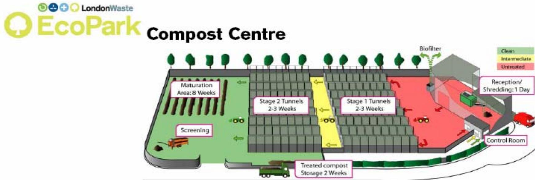
In the diagram above, the flow of material is from right to left. The process lasts about twelve to fifteen weeks from the point of reception to producing fully matured compost. On receipt, the waste is inspected to identify gross contaminants such as plastics, metals, glass and other undesirable items such as large logs and fence posts. The waste is then shredded and blended to reduce the particle size and produce a more consistent material that will compost more effectively.
