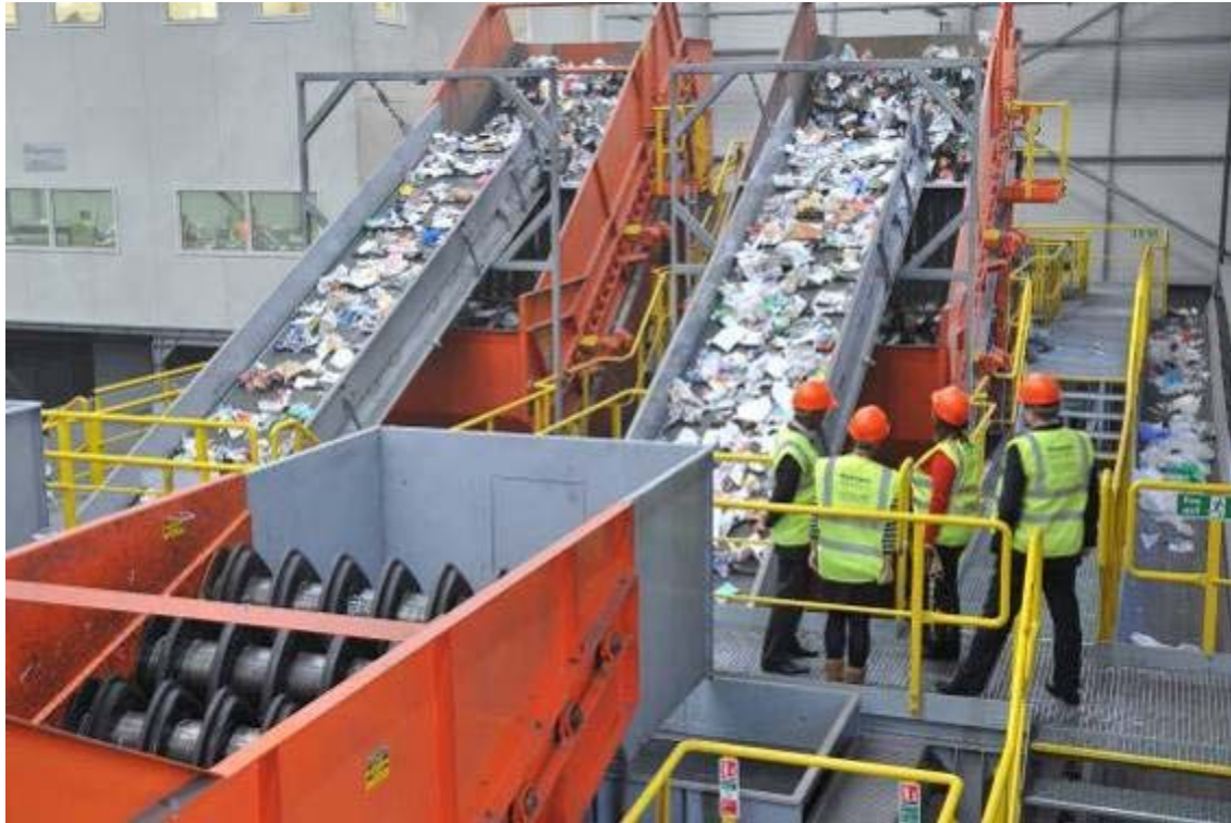
Mixed dry recyclable waste is sorted at a materials recycling facility (MRF).
