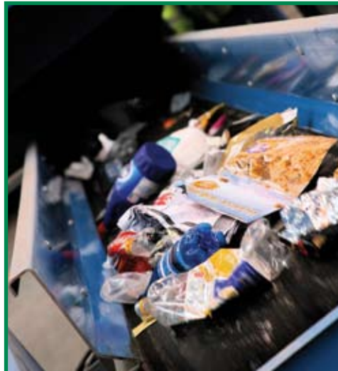
The in-feed area of a MRF
